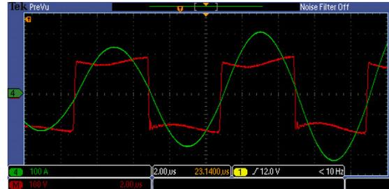
**Figure 3 – Optimally Tuned DRSSTC System**
