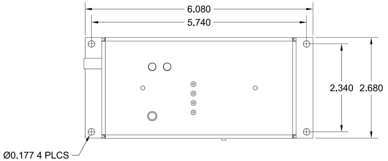
**Figure 11- Mounting Dimensions (inches)**
