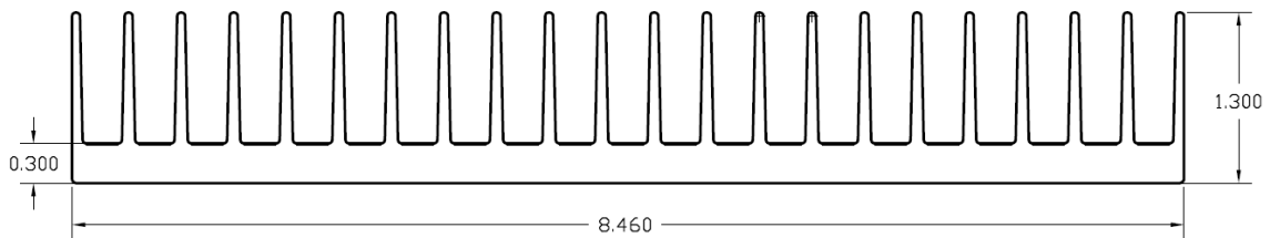
flexiBrute Heatsink 8.5 Profile (Thermal Impedance 1.10 °C/W/3.00")
